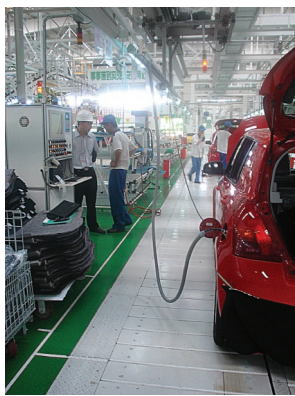
燃油系统气密及通气测试仪应用在汽车检测线上 Fuel system leak and ventilation tester applied to automobile detection line
